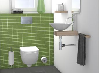
5) JACKOBOARD<sup>®</sup> Sabo must be covered with tiles to ensure the sufficiently even distribution of pressure when the WC is in use. The tiles can be laid directly on JACKOBOARD<sup>®</sup> Sabo. All types and sizes of tiles can be used in principle. The tiles should, however, measure at least 100 x 100 mm, and be at least 7 mm thick. Once the tile adhesive has hardened, the WC can be mounted on the tile surface.
