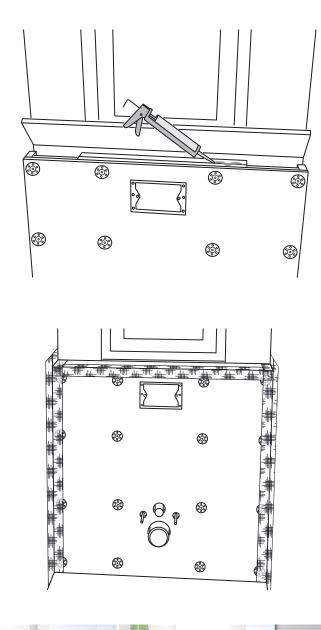
**3)** After cutting, the cover is bonded with a suitable assembly adhesive (e.g. JACKODUR<sup>®</sup> assembly adhesive, BOARD-FIX<sup>®</sup>).
