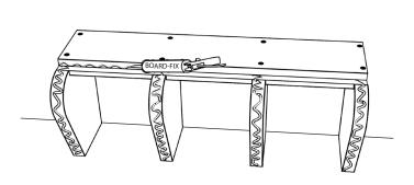
**7)** Apply BOARD-FIX® to supporting panels A and to the long side of cover B1.
