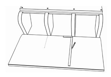
**6)** Fit cover B2 and mark the positions for the middle supporting panels.
