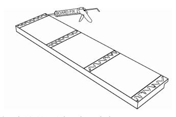
**3)** Apply BOARD-FIX® along the marked contours.
