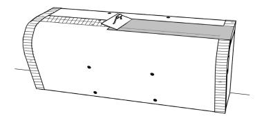
**14)** Apply tile adhesive over the glass fibre tape.
