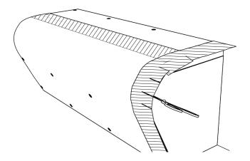
**13)** Tape over all butt joints and visible edges with JACKOBOARD® self-adhesive glass fibre tape. Cut into the glass fibre tape with scissors at the curves and glue on so that they overlap.
