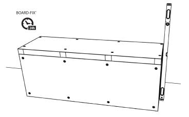
10) Glue the bench to the wall and the floor so that it is positioned upright
