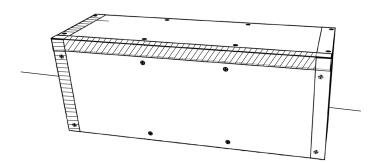
11) Tape over all butt joints and visible edges with JACKOBOARD® self-adhesive glass fibre tape.
