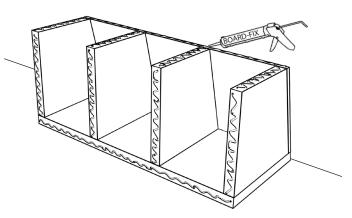
9) The bench must be glued to the wall and the floor. To do this, apply BOARD-FIX® to the front surfaces of the back and underside.
