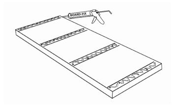
3) Apply BOARD-FIX® along the marked contours.
