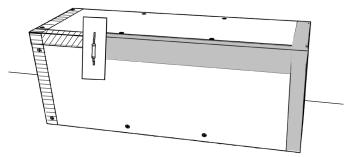
12) Apply tile adhesive over the glass fibre tape. The bench is now finished and can be tiled.
