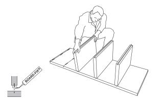
**3)** The shelves are glued on one after the other. The 80 mm shelf is positioned second from the bottom to match the washstand.
