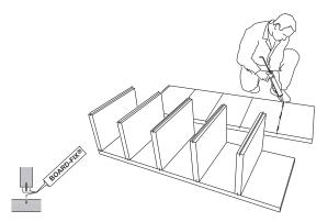
4) Apply adhesive to both joining parts (side wall and shelves).
