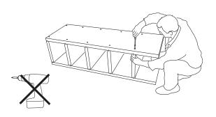
6) Screw both side walls of the unit tight by positioning the enclosed screws and washers in the pre-drilled holes. Using a manual screwdriver, tighten the screws until the heads are flush with the surface.
