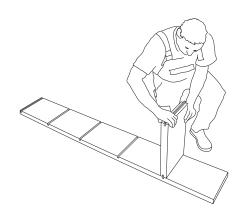
**2)** Insert the shelf into the groove on the side wall. Make sure the shelf and side wall are flush.
