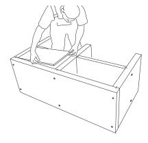
9) Press the former boards into the upper compartments of the washstand. They serve to keep it at right angles and are removed once the adhesive has hardened.
