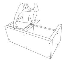
**9)** Press the former boards into the upper compartments of the washstand. They serve to keep it at right angles and are removed once the adhesive has hardened.
