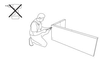
**3)** Screw the top to the side wall. To do this, position the screws and washers in the pre-drilled holes. Using a manual screwdriver, tighten the screws until the heads are flush with the surface.
