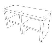
**10)** The washstand is now complete. Once the adhesive has hardened (approx. 24 hours) it can be directly covered with tiles or plaster. To ensure permanency, the washstand must be bonded to the base (wall and floor) using BOARD-FIX® adhesive. Please observe the following notes.
