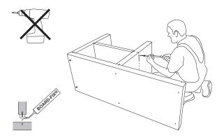
**5)** Once adhesive has been applied to all joining parts, screw the centre wall to the centre shelf.
