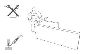
**4)** Apply adhesive to both joining parts (side wall and centre shelf) and screw on the centre shelf.
