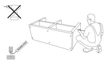
8) Apply adhesive to the 2nd side wall and screw it tight.
