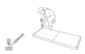
1) Apply adhesive to both joining parts (top and side wall).
