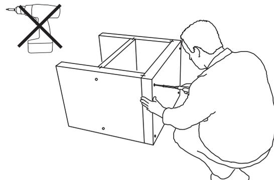
**6)** Screw the washstand together by positioning the screws and washers in all pre-drilled holes. Using a manual screwdriver, tighten the screws until the heads are flush with the surface.
