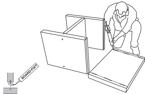
**4)** Apply adhesive to both joining parts (top and side walls).
