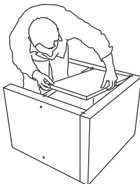
7) Press the former board into the upper compartment of the washstand. This serves to keep it at right angles and is removed once the adhesive has hardened.
