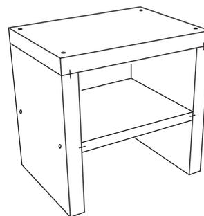
8) The washstand is now complete. Once the adhesive has cured (approx. 24 hours) it can be directly covered with tiles, filler or plaster. To ensure permanency, the washstand must be bonded to the base (wall and floor) using BOARD-FIX® adhesive. Please observe the following notes.
