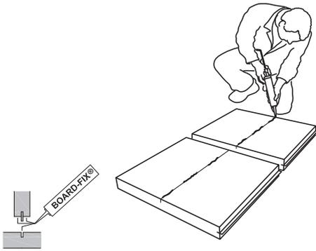
**1)** Apply adhesive to both joining parts (side walls and centre shelf).
