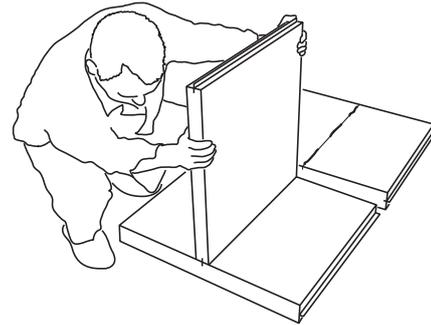
**2)** Insert the centre shelf into the groove on the side wall. Make sure the centre shelf and side wall are flush.
