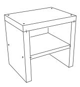
**8)** The washstand is now complete. Once the adhesive has cured (approx. 24 hours) it can be directly covered with tiles, filler or plaster. To ensure permanency, the washstand must be bonded to the base (wall and floor) using BOARD-FIX® adhesive. Please observe the following notes.
