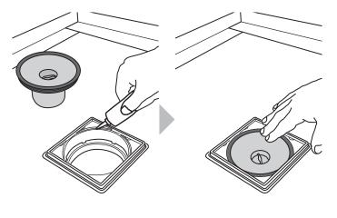
**10)** Grease the top edge of the top piece (8) with installation grease (1 packet of installation grease is included in the box containing the drain). Then insert the odour trap (6)
