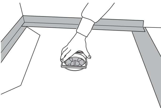
**11)** Cut the top piece (4) to the right length to match the thickness of the tiles, and position in place. Use tile adhesive in the four corners to adjust the top piece (4) to exactly the right height.
