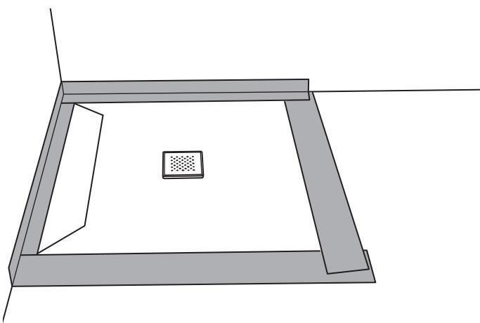
**12)** Position the grate (3) in place. The shower element is ready for tiling.
