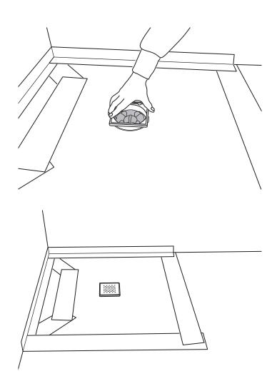
11) Cut the top piece (4) to the right length to match the thickness of the tiles, and position in place.Use tile adhesive in the four corners to adjust the top piece (4) to exactly the right height.
