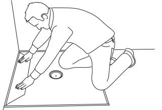
**8**) Position the pipe duct element (2) in the screed recess and press firmly into place. BOARD-FIX<sup>\*</sup> (6) special adhesive and sealing agent guarantees the durable seal integrity of the bond.
