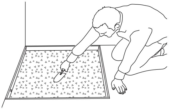
**2)** Apply tile or flexible adhesive with a notched trowel to the underside of the shower element.
