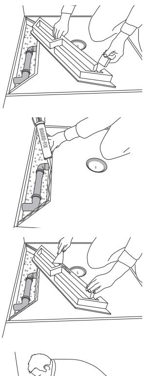
**5)** On the underside of the pipe duct element (2) the break-throughs for the waste pipe be made with a cutter.
