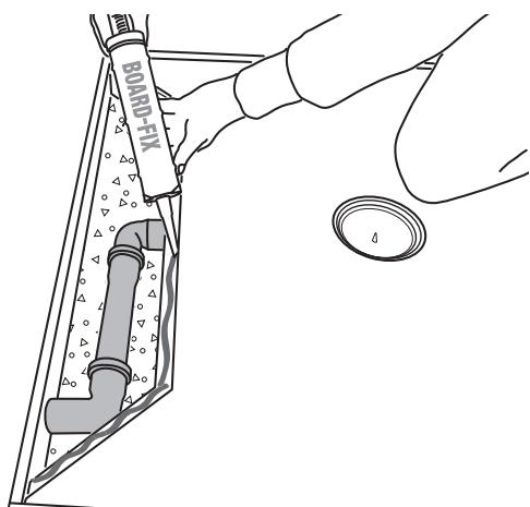
**6)** Apply the BOARD-FIX® (6) special adhesive and sealing agent in beads to the shiplap on the shower element. Make sure the adhesive is applied consistently, with no interruptions.
