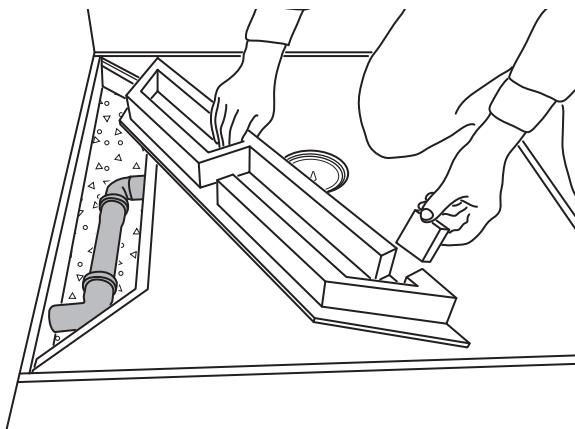
**5)** On the underside of the pipe duct element (2) the breakthroughs for the waste pipe be made with a cutter.
