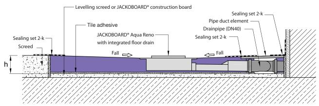
Min. installation height (h) = JACKOBOARD® Aqua Reno (65 or 75 mm) + 5 mm tile adhesive
