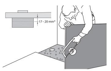
\*12 - 15 mm into the drain bowl + 5 mm bonding mortar
