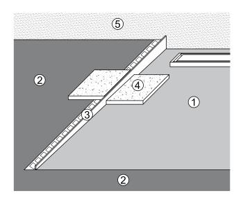
The sloping JACKOBOARD<sup>®</sup> Aqua Line Profile (available as an accessory) can be inserted between the edge and the screed. The sloping profile is available as a left version (illustrated) or as a right version.
