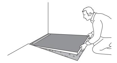
**7)** Position JACKOBOARD<sup>®</sup> Aqua Line pro in the screed recess, making sure the drain nozzle on the channel fits into the seal ring on the drain.
