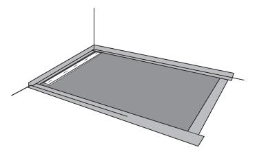
**10)** Once Installation of JACKOBOARD® Aqua Line easy is finished the shower element can now be tiled.
