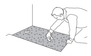
**6)** Remove the protective cover. Apply cement-based single part flexible tile adhesive to the entire underside of the shower board.
