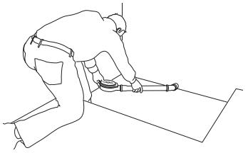
4) Insert the floor drain into the existing DN 50 pipe. Make sure the drain is at the right height and position (see the illustration "Installation height", Pages 6 and 7). In the case of floor structures with impact sound insulation, include the installation of suitable impact sound insulation and edge insulation strips in the planning.
