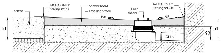
h1 = 148 mm (Minimum installation height for 40 mm shower element thickness)
