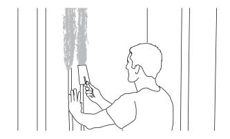
**11)** All longitudinal joints on the inner side of the wall elements are reinforced with JACKOBOARD® reinforcement tape and filled using tile adhesive. The top edges at the entrance and the lengthwise joints on the outside are also filled with JACKOBOARD® glass fibre tape.
