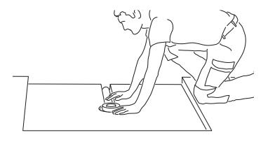
**5)** The base of the floor drain is pushed into the DN 50 discharge pipe...
