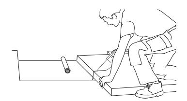
**3)** Cement based single part flexible adhesive is applied to the underside of the base element with a notched trowel.
