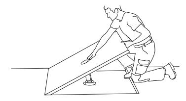
**7)** The shower element is bonded to the base element using cement based single part flexible adhesive using a 5 cm notched trowel applied to the entire surface.
