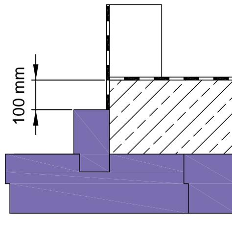
Waterproofing direction on building site according to DIN 18533
