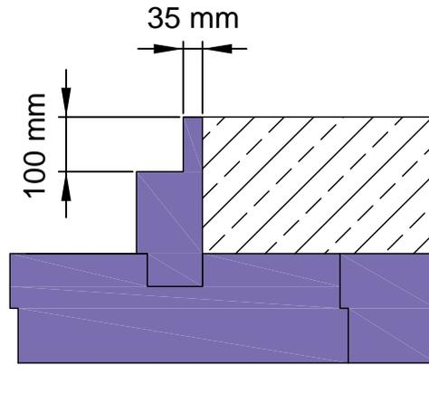
Formwork element for Waterproofing (with 35 mm foam edge).
