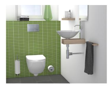
6) JACKOBOARD<sup>®</sup> Sabo Assembly Set must be covered with tiles to ensure the sufficiently even distribution of pressure when the WC is in use. The tiles can be laid directly on JACKOBOARD<sup>®</sup> Sabo Assembly Set. All types and sizes of tiles can be used in principle. The tiles should, however, measure at least 100 x 100 mm, and be at least 7 mm thick. Once the tile adhesive has hardened, the WC can be mounted on the tile surface.
