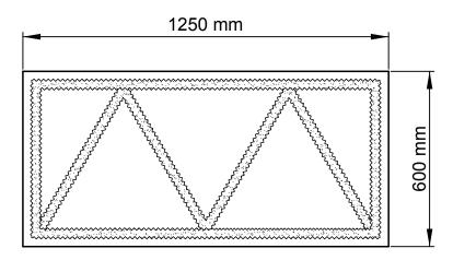
**Dowelling** with JACKODUR® Etics anchors, 4 anchors/board (0,75 m<sup>2</sup>)
