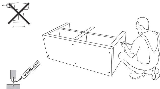
8) Apply adhesive to the 2nd side wall and screw it tight.
