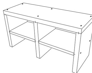
10) The washstand is now complete. Once the adhesive has hardened (approx. 24 hours) it can be directly covered with tiles or plaster. To ensure permanency, the washstand must be bonded to the base (wall and floor) using BOARD-FIX® adhesive. Please observe the following notes.
