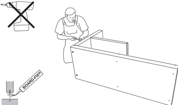
4) Apply adhesive to both joining parts (side wall and centre shelf) and screw on the centre shelf.
